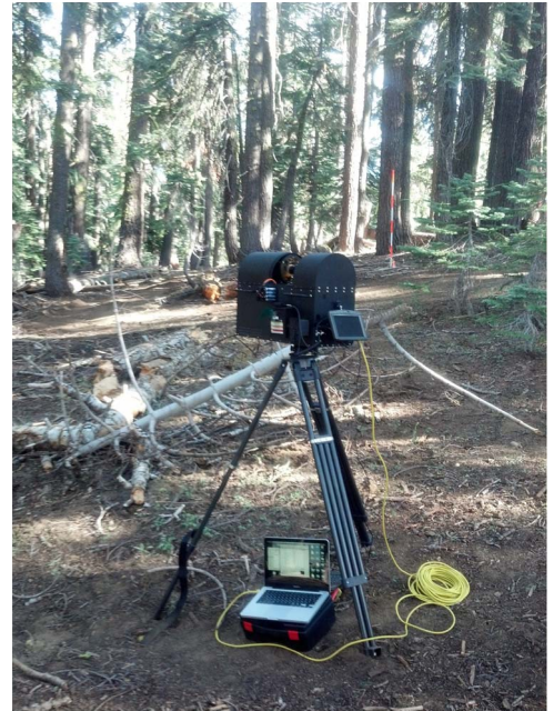
Fig. 4. Complete DWEL instrument deployed in the Sierra Nevada National Forest, before the case was painted bright orange.
