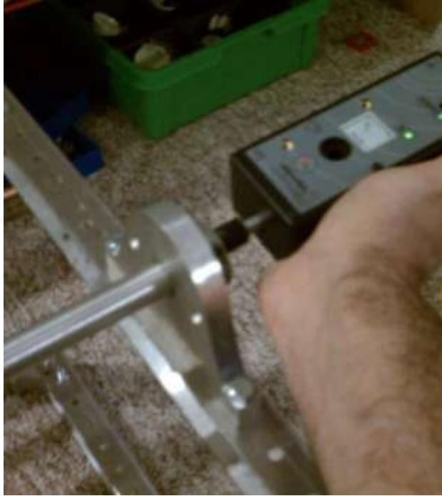
Figure 27: Application of Lateral (Axial) Force on Pendulum Rod
